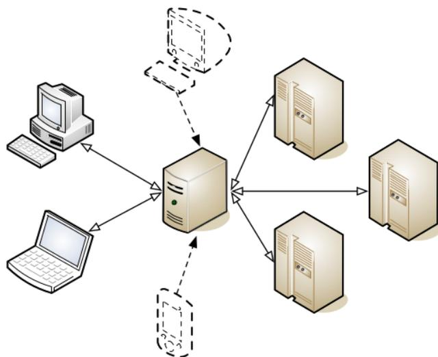
Use the JobServer & TaskServer as a gateway for high performance computing in computer centers or the cloud. The JobServer & TaskServer support the most common load balancing systems such as SLURM, PBS/Torque, and GridEngine.
