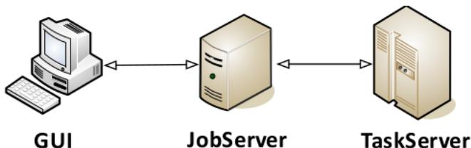
For smaller compute clusters, easily install a single central JobServer on a dedicated machine, and install TaskServers on the compute nodes. With this setup, submit calculations from one or more computers, which have the MedeA GUI's installed. MedeA's JobServer & TaskServer have web interfaces to manage and monitor jobs, and restrict access if necessary.
